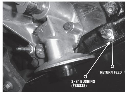
3. Remove the plugs and insert hose fittings (FMAL). The port on the left of the OE filter base will be the pressure feed. The return feed will be on the right. Use 3/8" bushing (FBUS38) in return feed, pictured below.
